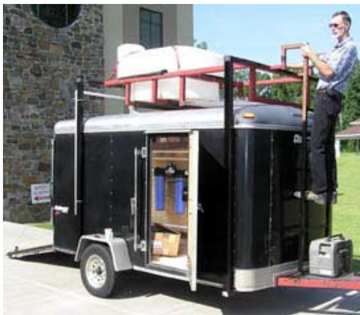
Advent Church's Floyd Graves examines the new trailer, which contains two complete standard water treatment boards on slide-out stands. The vehicle is designed for emergency and training use.
