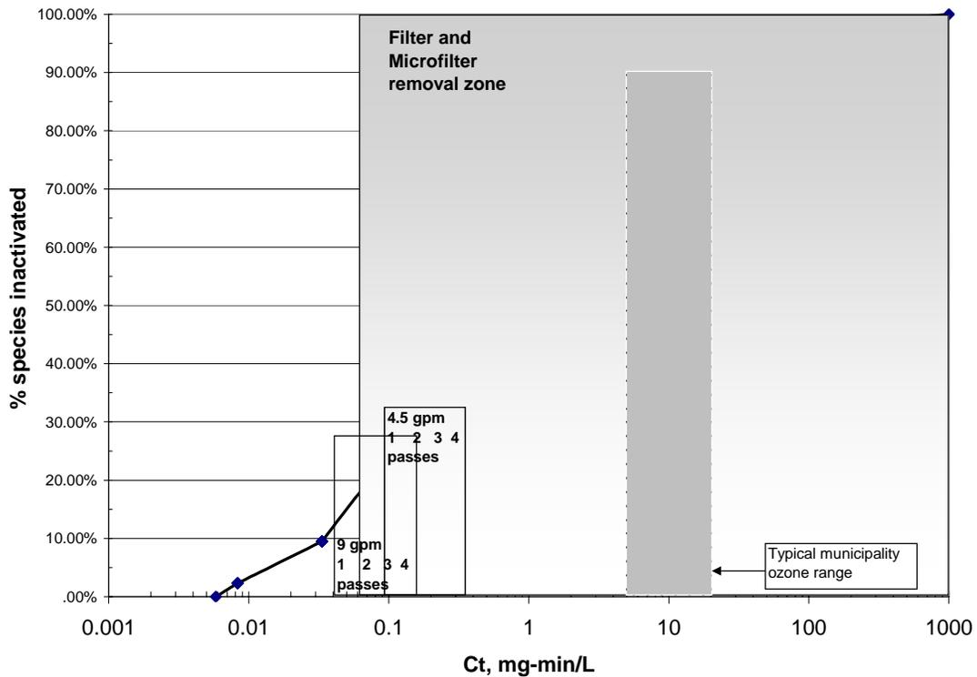
The PZII-2 ozone generator has a set ozone delivery rate of 1 g/hr, so, unlike bleach where more can be added, we can't increase the dose the PZII-2, since the two lamp cartridges fix its ozone production rate. However, Prozone manufactures a PZII-4 that would double the amount of ozone dosed to the system, and larger arrays of lamp cartridges are also available.
