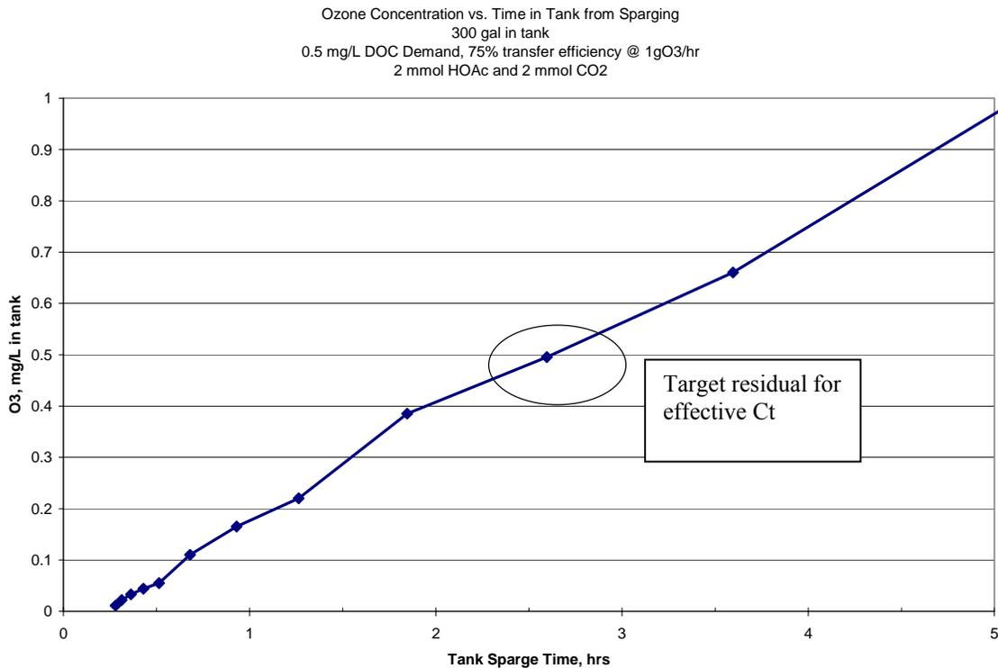
Under these premises, it will take approximately 30 minutes to react with the organic carbon, and then a total of 2.5 to 3 hours to build up to 0.5 mg/L ozone concentration, which is recommended by NSF.<sup>5</sup>
